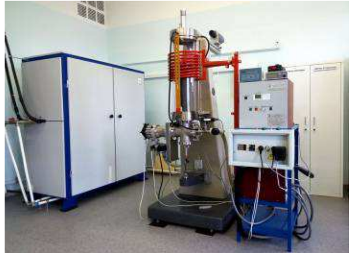
Fig. 2. System for growth of graphene films on SiC
