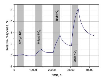
Response on exposure to the gas mixture containing  $NO_2$  in concentrations: 0.2 ppb, 0.5 ppb, 1 ppb and 2 ppb at  $110^{\circ}$ C. Exposure periods are shown as grey band.
