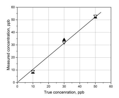
$NO_2$  concentration measured by graphene sensor versus true concentration measured by Apna 360 Horiba Scientific chemiluminescence analyzer. Black triangle correspond to the result of the first measurement cycle, white triangles to the second measurement cycle, and the solid line is linear approximation.
